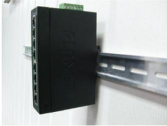
**Step 3:** Make sure the DIN-rail bracket is tightly on the track.
