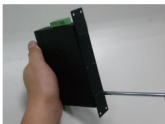
**Step 3:** Use the screws to screw the wall-mount plate on the Industrial Media Converter.
