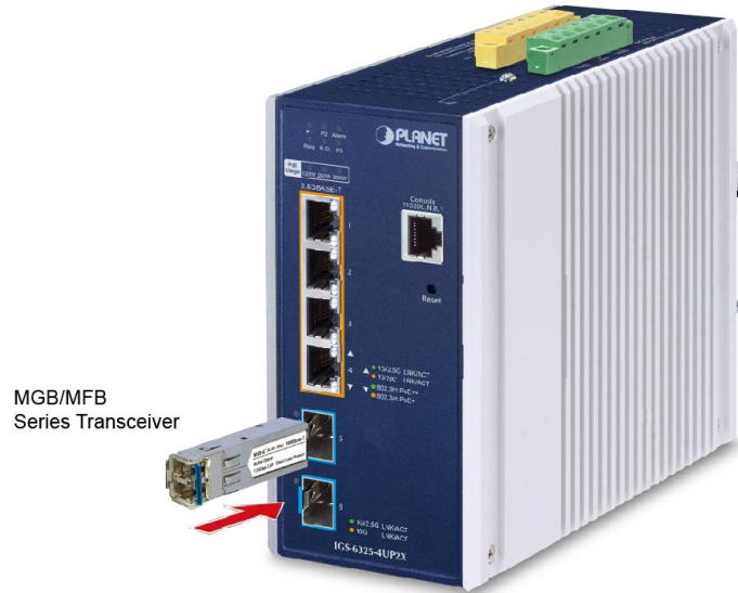
Figure 2-11: Plug in the SFP/SFP+ Transceiver
