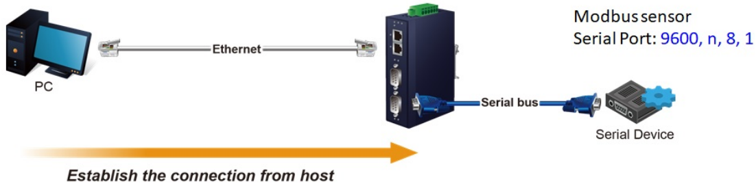
Figure 4-5-17: TCP Server Mode Application
