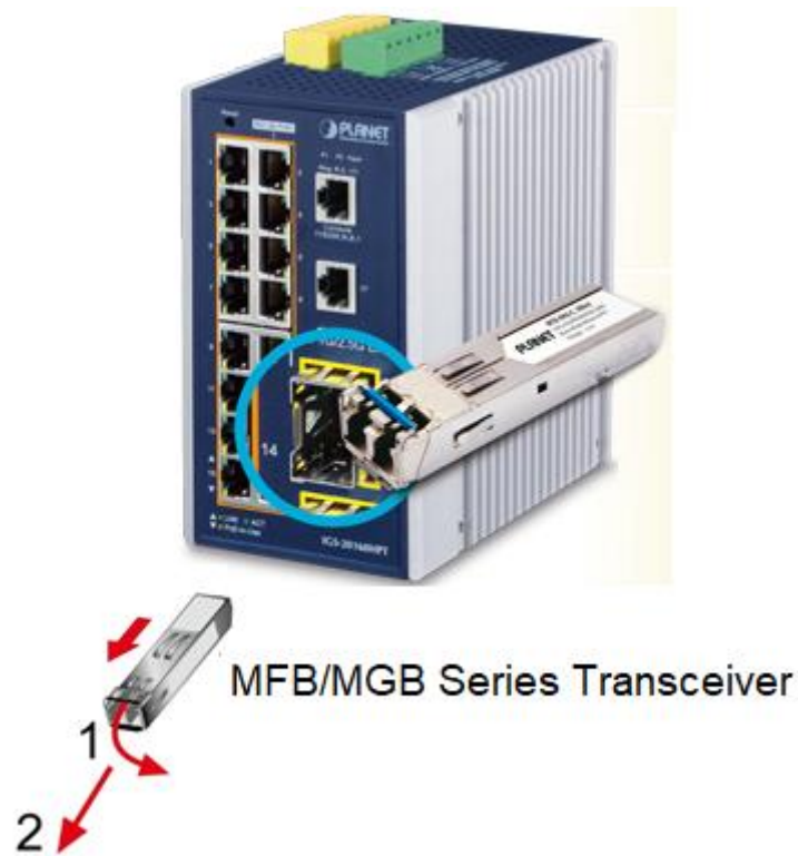
Figure 2-3-2: Pull out the SFP/SFP+ Transceiver Module
