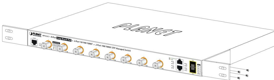
Figure 2-1-5 Attach Brackets to the LRP Managed Switch.
