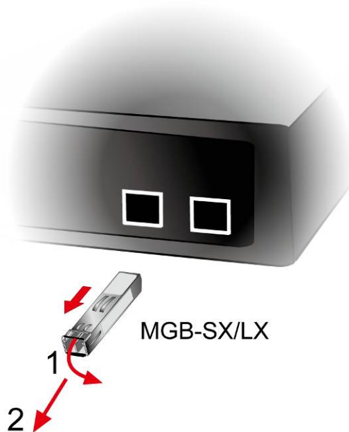
Figure 2-1-8 How to Pull Out the SFP Transceiver
