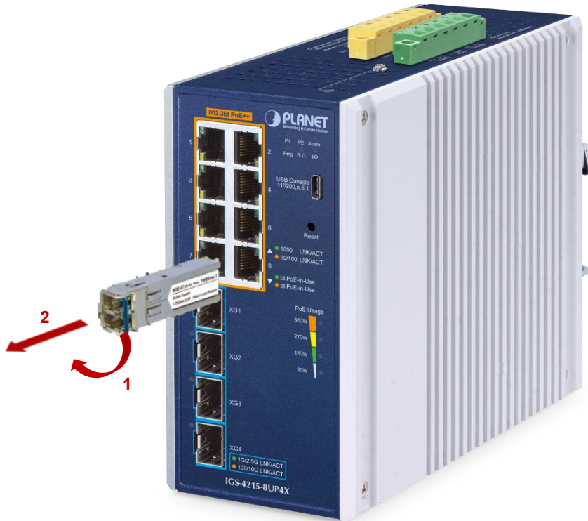
Figure 2-2-5: Remove the SFP Transceiver Module
