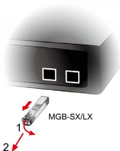
Figure 2-1-2g How to Pull Out the SFP Transceiver
