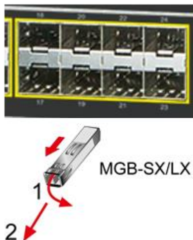
Figure 2-6 Pulling out the SFP/SFP+ transceiver
