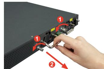
Figure 5-1 Removing the GPL-PWR75-DC
