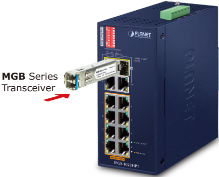
Figure 3-1: Plugging in the SFP Transceiver
