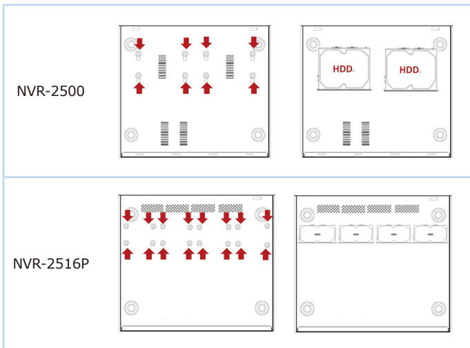
Figure 3-1: Hard Disk Installation
