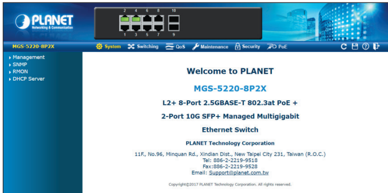
Figure 4-3: Web Main Screen of Managed Switch
