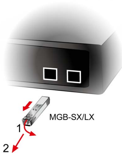
Figure 2-2-5: How to Pull Out the SFP/SFP+ Transceiver
