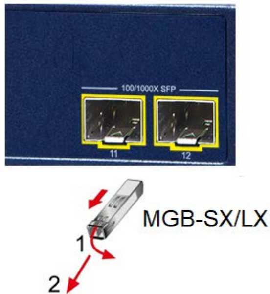
Figure 2-2-5: Pull out the SFP transceiver
