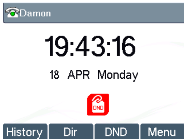
Figure 57 - DND Enabled on All Lines
