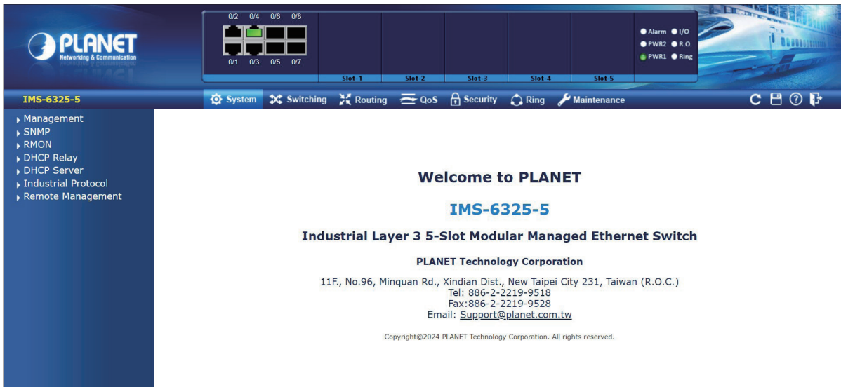
Figure 5-5: Web Main Screen without Installed Expansion Cards
