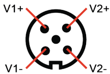
M12 DC power cable pin assignment & wire code
