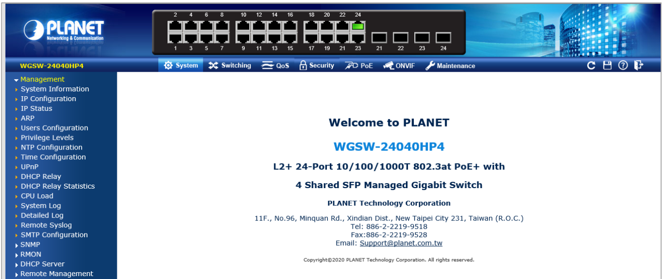
Figure 4-1-5: Managed Switch Main Functions Menu
