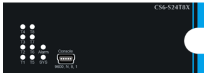
Figure 2-8 CS6-S24T8X LED Panel
