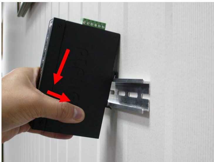
Step 2: Lightly press the button of DIN-Rail into the track.
