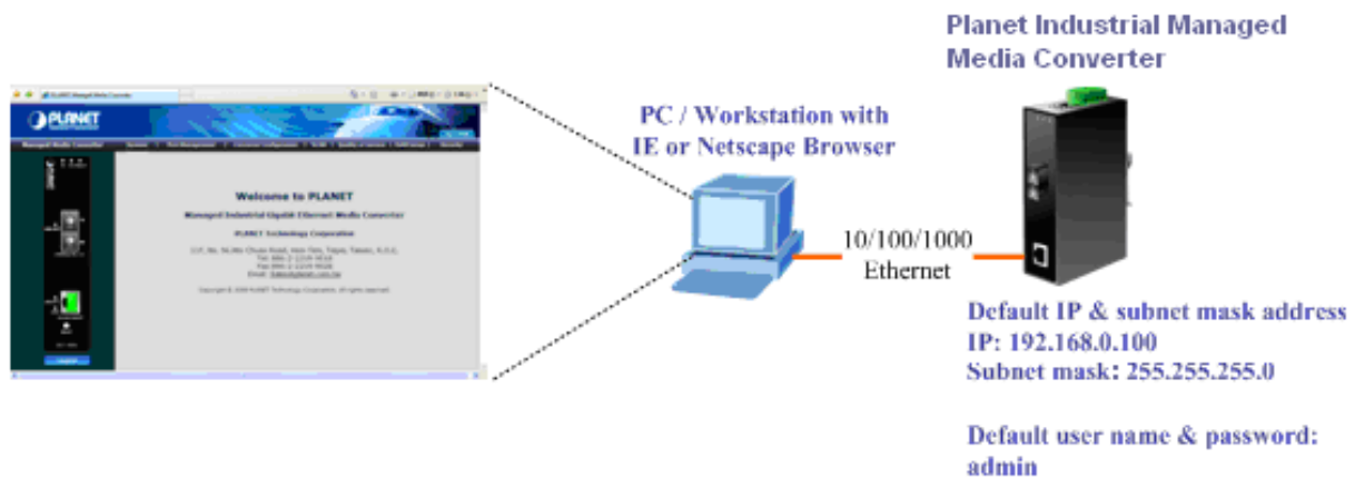
Figure 3-1 Web Management over Ethernet
