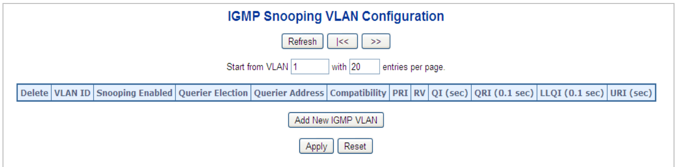
Figure 4-8-8: IGMP Snooping VLAN Configuration Page Screenshot
