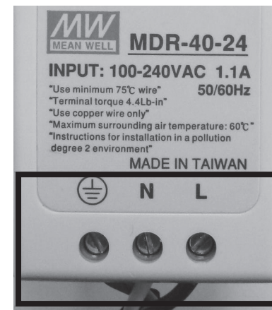
Figure 1. Connecting the 3 wires to the corresponding location.
